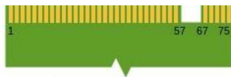
Figure 5-2 M.2 PCIe SSD Pin Assignment
